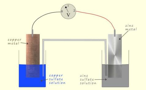
a. In this cell the zinc metal reduces the copper ions present.
